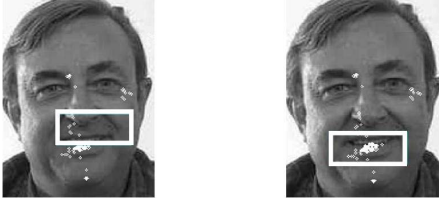
Figure 6. Illustration of difference between maximum likelihood and maximum density approaches. Left: maximum likelihood estimation. Right: maximum density-based robust consensus voting using mean shift. White dots indicate center locations of root candidates F_{mn} for mouth case.
