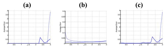
Figure 6: Average variance estimation errors of the most-stable-over-scales methods over 100 independent tests. The same types of data in Fig.3 with different random noise are used for each test. The errors are plotted against varying sampling ranges. Dot and solid lines denote errors by the first- and the second-order methods, respectively.
