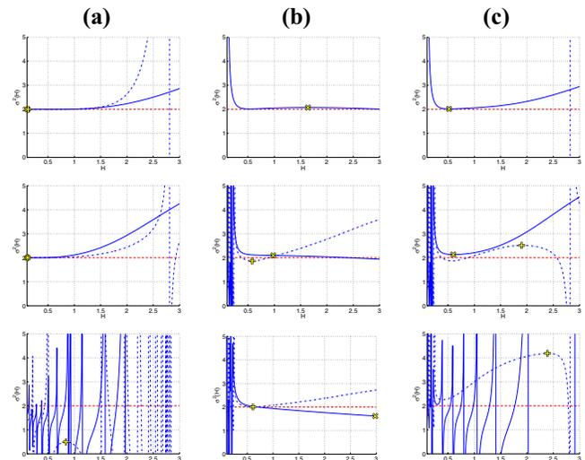
Figure 5: Variance estimation by the most-stable-over-scales methods for the signals in Fig.3. At each analysis scale, the variance of the target is estimated from samples within: 1st row:  $\pm 0.1\sigma$ , 2nd row:  $\pm 1.0\sigma$ , 3rd row:  $\pm 2.0\sigma$ . The legend is the same as Fig.2.
